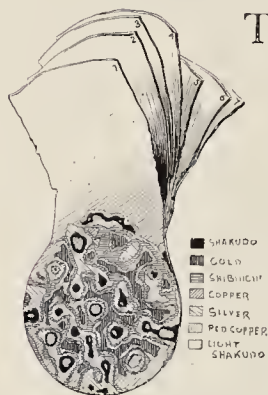
Fig. 1.—Illustration of method of blending alloys.
